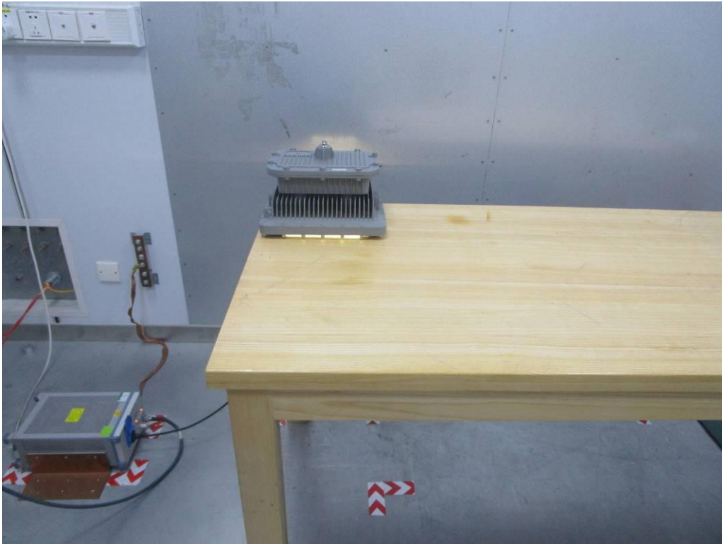
Conducted Emissions test setup photo
